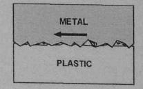
surfaces and this results in one part actually floating over the other. The two articulating surfaces do not come into contact if the parts are moving. Also, the bearing is usually moving at a constant velocity and in a unidirectional motion. Under these conditions, abrasive wear is negligible. In the body, the motion is oscillating and the liquid film cannot be maintained.
